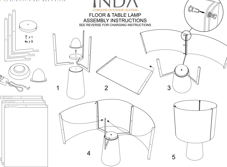
IF ADDED WEIGHT IS DESIRED FILL WITH SAND WITH FUNNEL THROUGH HOLE ON TOP OF BASE BEFORE ASSEMBLY
